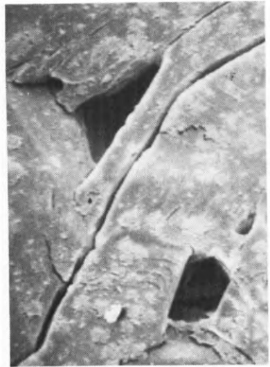
Flaked, Cycled Twice at 150°C, 5°C/min
