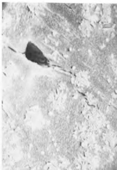
Flaked, Cycled Twice at 150°C, 5°C/min
